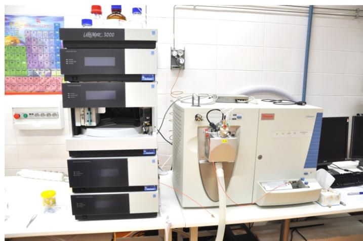
Dionex Ultimate 3000 UHPLC system together with LCQ Fleet mass spectrometer
